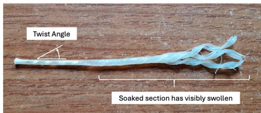
Figure 4. Section of gut string. The ‘twist angle’ is defined as the angular deviation of the twisted string from the untwisted case. Reproduced from [38], AIP, 2021.
